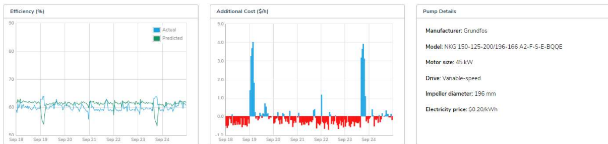
Figure 2: The efficiency of a pump is modelled out vs the manufacturers efficiency curve, and a cost to run is attributed through the resulting performance.
