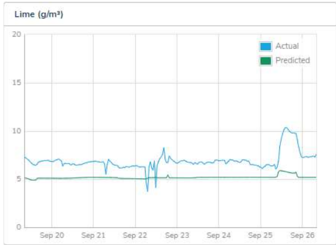
Figure 4: Tracking chemical usage against expected or predicted values offers insights into reduce plant performance.
